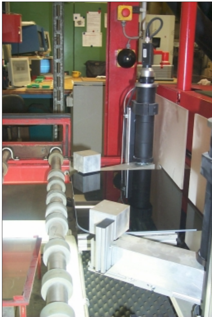
Inspection of ground edges in a production line for automotive glass
