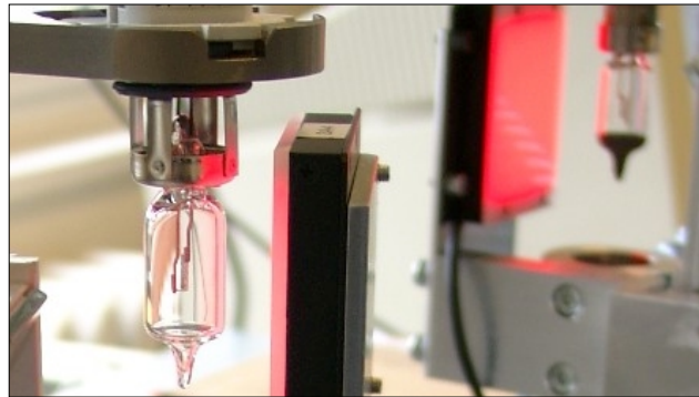
Lamps in the inspection station
